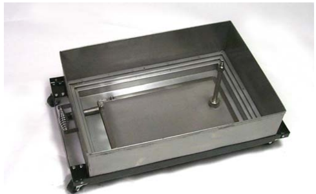
Filter leaf properly positioned in filter pan.
